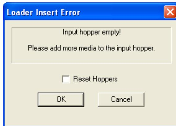
In this example, there is a Reset Hoppers check box. If checked, this tells the robot to start taking blank media from the first hopper again. If this box is not checked, the robot will continue picking from the last hopper used.
